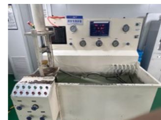
Pressure Test for Large Valve
