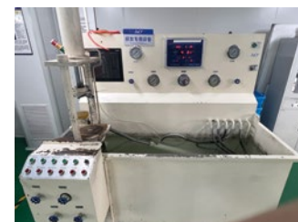
Pressure Test for Large Valve
