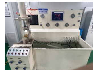
Pressure Test for Large Valve
