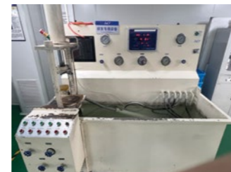
Pressure Test for Large Valve
